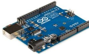
**Fig-3:** Arduino Board
