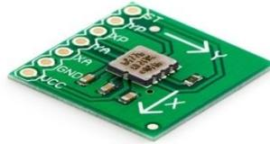
**Fig -2:** Accelerometer
