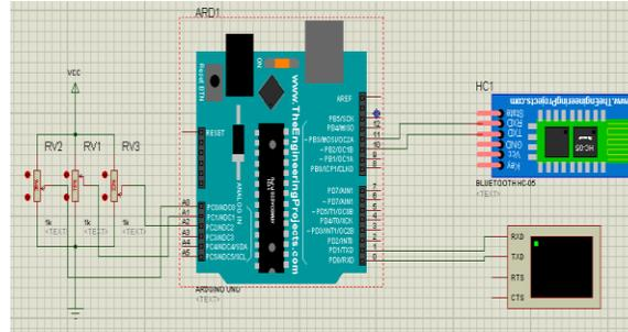
Fig-7: Interfacing Diagram
