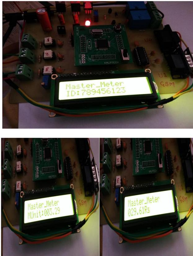
Fig.8: LCD display meter ID ,consumed unit and bill
