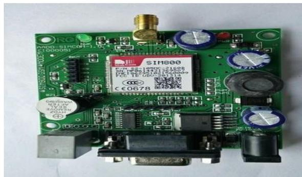
Fig 2: GSM Module
